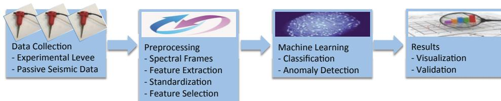
Figure 2: General data processing and anomaly detection workflow.
