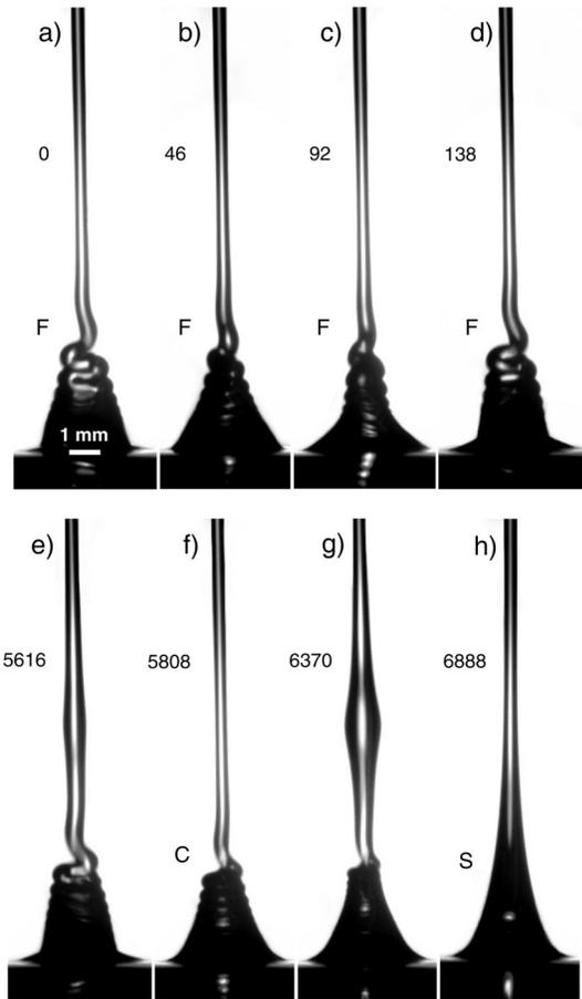
FIG. 1. Time sequence of photographs showing three possible states of a viscous column with  $\nu = 946$  cS,  $Q = 0.19$  ml/s,  $d = 2.6$  mm, and  $H = 14$  cm. (a)–(d) Folding with rotation, (f) steady coiling, (h) axisymmetric stagnation flow. Panels (e) and (g) show the finite-amplitude perturbations that trigger the transitions between states. Numbers indicate time in ms.
