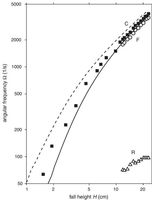
FIG. 4. Angular frequencies of coiling ( $C$ , solid squares), folding ( $F$ , open circles), and rotation of the folding plane ( $R$ , open triangles) as a function of height for an experiment with  $d = 2$  mm,  $\nu = 946$  cS, and  $Q = 0.132$  ml/s. Solid line: Numerical prediction of the coiling frequency using the method of [6]. Dashed line: Same, but without surface tension.
