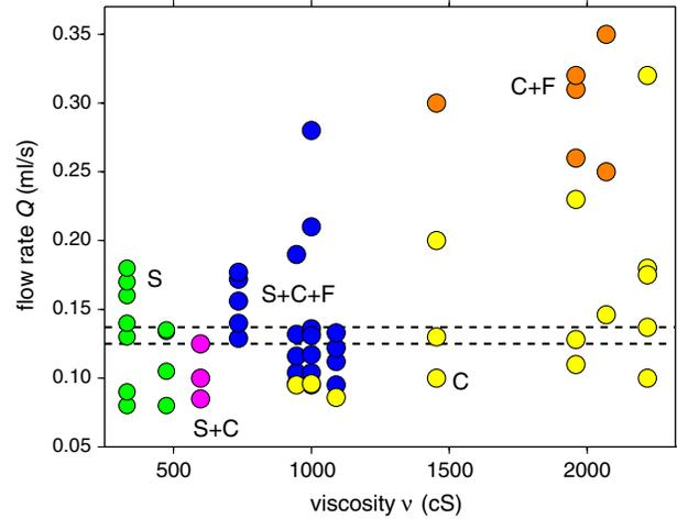
FIG. 2 (color online). Experimentally determined phase diagram in the space  $(\nu, Q)$ . In most cases, the hole diameter was  $d = 4$  mm for  $\nu \geq 1450$  cS and 2 mm for  $\nu \leq 1090$  cS. Experiments with  $\nu = 1000$  cS using both hole sizes confirm that the phase diagram is independent of  $d$ . The dashed lines indicate the range of values of  $Q$  used in Fig. 3.
