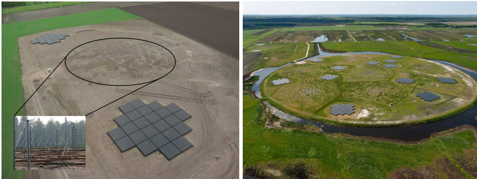
Figure 1.2: Left: Aerial photo of a LOFAR core station on the superterp near Exloo, the Netherlands. A core station consists of two HBA fields made up of 24 tiles, a tile being an assembly of 16 HB Antennas arranged on a 4 \times 4 grid, and one LBA field with 96 LB Antennas (see inset). Right: An aerial photo of the LOFAR superterp with diameter of 340 m and its 6 core stations. The superterp is located in the heart of the LOFAR core area, having a diameter of 2–3 km and containing 22 core stations. Photo credits: ASTRON.
