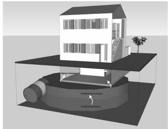
Fig. 1 Overview vapour intrusion from the contaminated source
