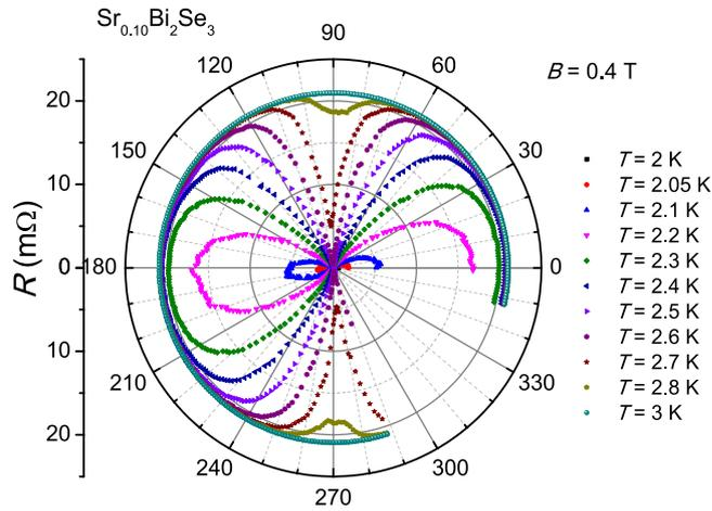
**Figure 2. Polar plot of the resistance of  $\text{Sr}_{0.10}\text{Bi}_2\text{Se}_3$ .** Resistance of  $\text{Sr}_{0.10}\text{Bi}_2\text{Se}_3$  as a function of angle  $\theta$  in a magnetic field of 0.4 T and temperatures ranging from 2.0 K to 3.0 K presented in a polar plot. The angle  $\theta = 3^\circ$  corresponds to  $B \parallel a^* \perp I$ , while  $\theta = 93^\circ$  corresponds to  $B \parallel a \parallel I$ .
