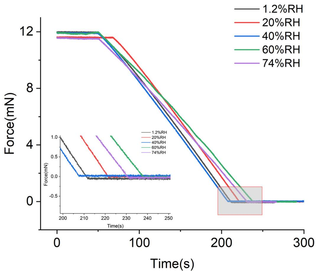
FIG. S3. Force as a function of time measured during the retraction of a sphere from a worn sphere at a speed of 77 nm/s till the surfaces were separated, the inset shows the force near the contact separation point.
