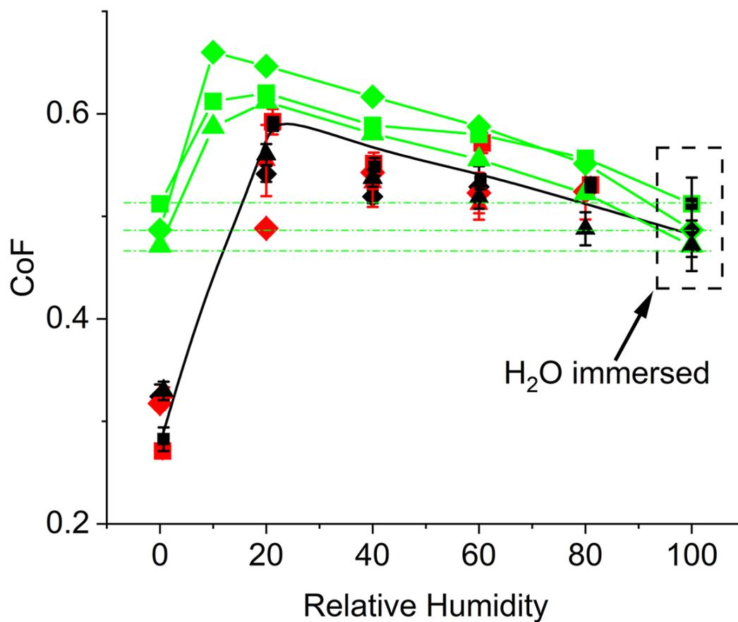
FIG. S4. Calculated and measured coefficient of friction as a function of relative humidity. The red and black symbols indicate friction experiments conducted at increasing (black) and decreasing (red) relative humidity varying from 0.6% to 80%. Squares, triangles and diamonds each correspond to an experiment conducted with a different sphere. The corresponding simulation results are represented by matching green symbols.
