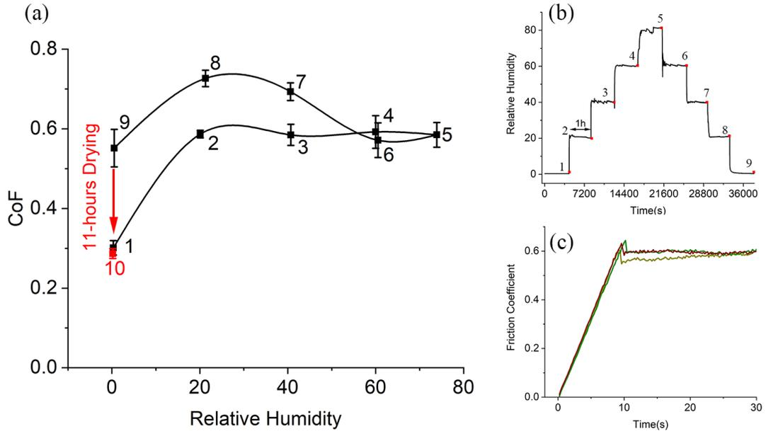
FIG. S1. Friction coefficient hysteresis loop as a function of relative humidity (a). In total ten sets of friction experiments were performed. The corresponding humidity-time curve and the times at which friction experiments were conducted are marked with red dots and numbers in (b). (c) is one example of how the friction coefficient is defined in the steady state at 20% humidity.
