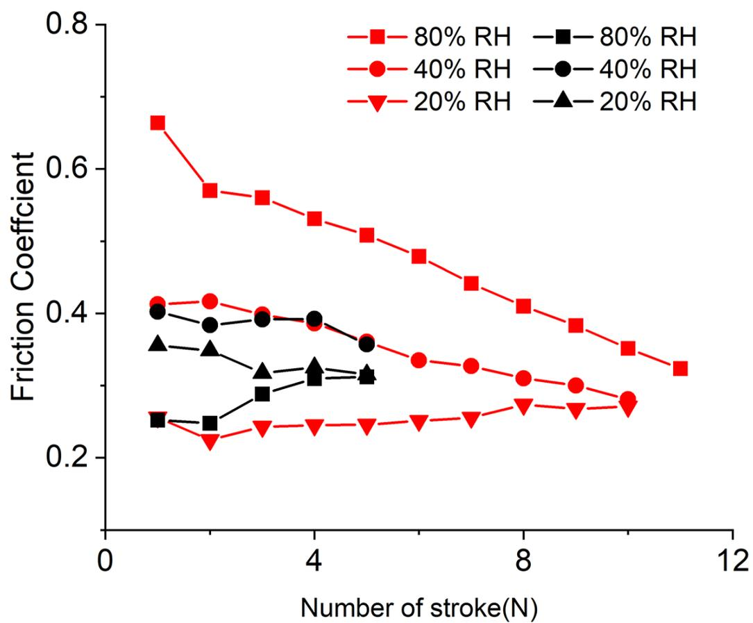
FIG. S2. Friction coefficient as a function of the number of strokes measured after drying the system for one hour. The black solid and red solid lines indicate the situation with (black) and without (red) contact separation after sliding in a specific humidity environment.
