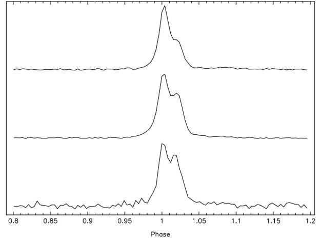
**Fig. 1.** Standard profiles for the three different frequencies used at Westerbork. From top to bottom: 840 MHz, 1380 MHz, 2300 MHz. The effective time resolution ( $102.4 \mu$ s) is similar to the size of one bin ( $160 \mu$ s).
