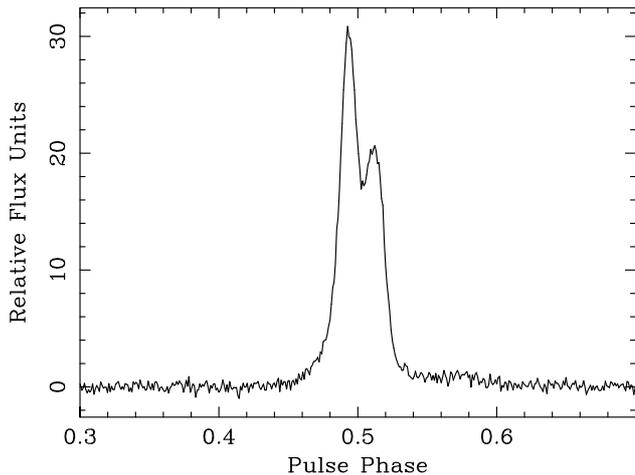
**Fig. 8.** A pulse profile obtained using PuMa II at the WSRT. The data were obtained in a 30 min observation at 1380 MHz with a bandwidth of 160 MHz and were analysed using a coherent filterbank with 512 frequency channels and a time resolution of  $6.4 \mu\text{s}$ . A similar pulse phase range is shown as in Fig. 1 and the improved resolution shows somewhat more detail in the pulse profile.
