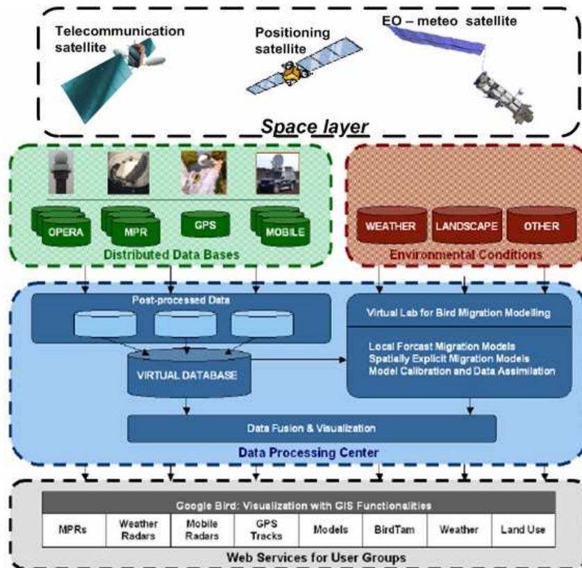
Figure 3: Flysafe system of systems overview. The Flysafe system concept exhibit four main elements: sensors; data collection network; data storage, post-processing and modelling; and data distribution and visualization.
