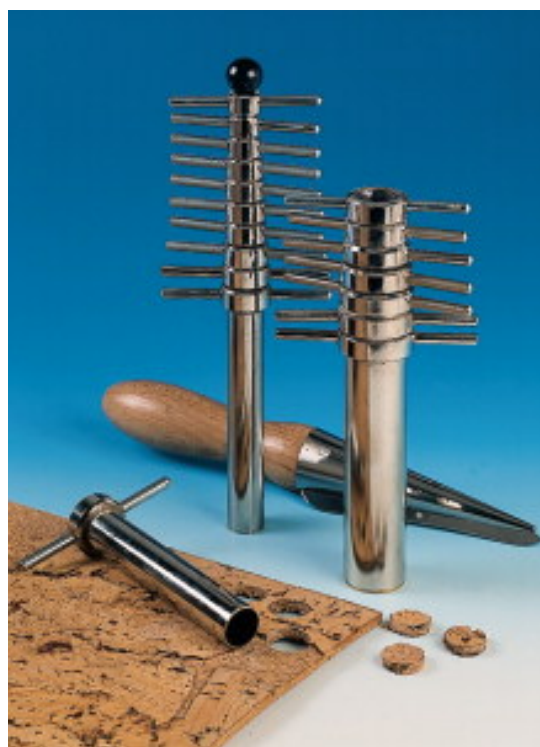
Example of a cork corer, which can be used to sample volumetrically from peat (photo courtesy of Carl Roth GmbH + Co. KG).
