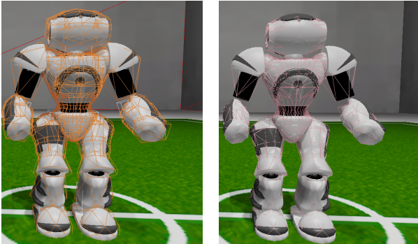
Figure 3: The left picture shows the PhysX collision model, the right picture the Unreal Engine collision model.
