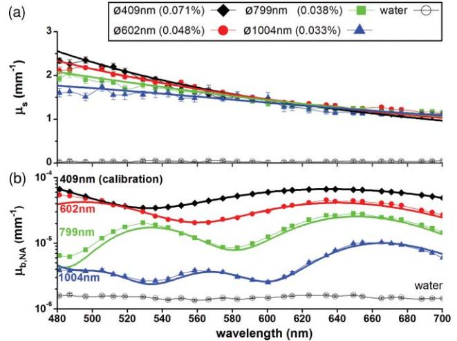
**Fig. 1** LCS (dots) and Mie (thick solid lines) results for (a) scattering coefficients  $\mu_s$ , and (b) backscattering coefficients  $\mu_{b,NA}$  for four aqueous suspensions of different sized polystyrene spheres and water. Error bars, representing the 95% c.i. of the fitted values, may fall behind data points. The  $\mu_{b,NA}$  were calibrated using the 409-nm sample.
