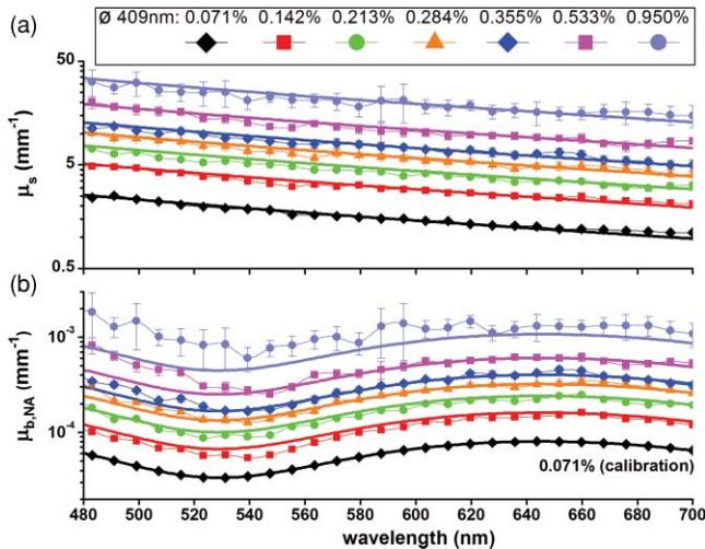
**Fig. 2** LCS (dots) and Mie (thick solid lines) results for (a) scattering coefficients  $\mu_s$ , and (b) backscattering coefficients  $\mu_{b,NA}$  for six concentrations of 409-nm polystyrene sphere suspensions. Error bars, representing the 95% c.i. of the fitted values, may fall behind data points. The  $\mu_{b,NA}$  were calibrated using the 0.071% sample.
