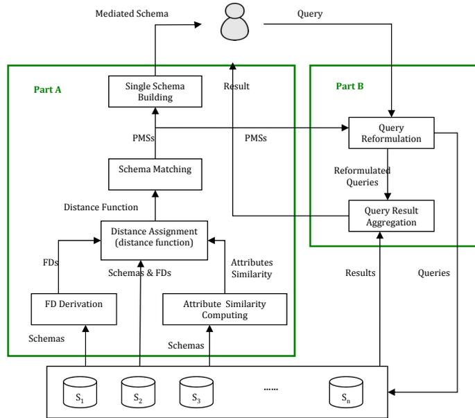
**Fig. 1.** Architecture of our data integration system
