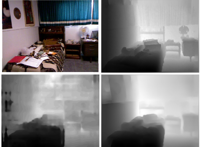
Figure 6. Depth estimation examples. Left top: input image. Right top: ground truth. Left bottom: predicted depth by DORN [10]. Right bottom: prediction by our D-DFN. Prediction by DORN shows artifacts and the local depth edges or gradient consistency are not well recovered, while our D-DFN output much sharper local depth structure.
