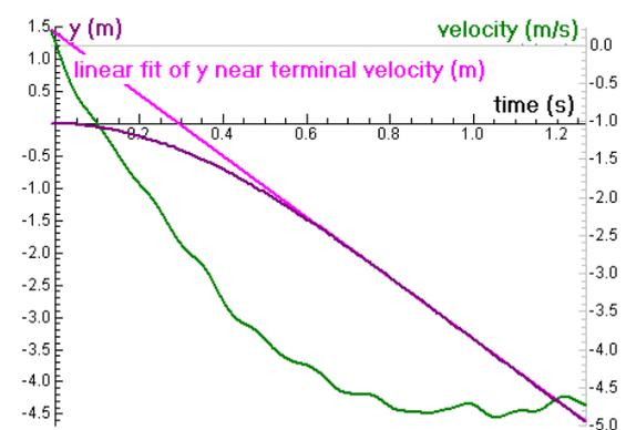
**Fig 3.** The vertical position-time graph (purple curve) and the velocity-time graph (green curve) of the falling shuttlecock. The linear function fit of the position-time graph shows the approach to linear motion after about 0.8 second.
