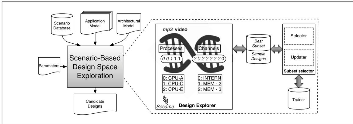
**Figure 7. The exploration framework for scenario-based DSE.**
