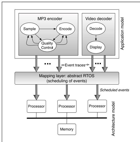
**Figure 4. The Sesame system-level MPSoC simulation infrastructure.**
