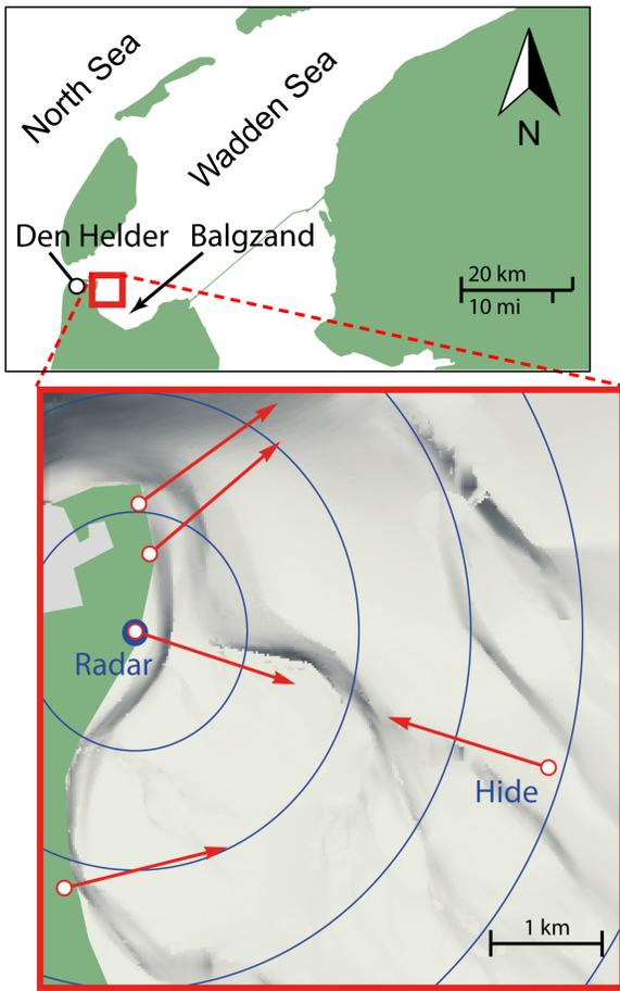
**Figure 1. Study area and position of the bird radar.** Map of the north-western part of the Balgzand intertidal area in the Wadden Sea, the Netherlands, showing the position of the radar (blue dot) and the transects used by visual observers (red arrows into the direction of observation). Concentric circles around the radar position are separated by a range of 1 km.
