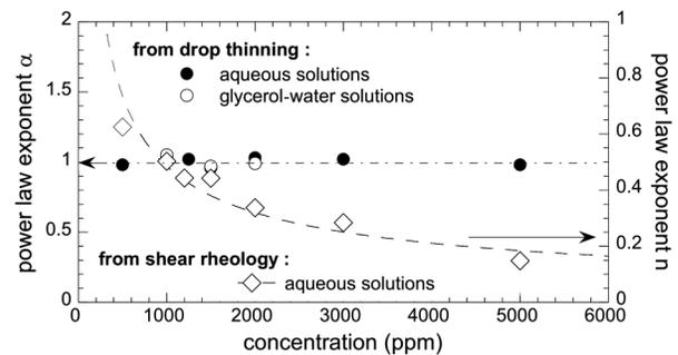
FIG. 6. Left scale: power-law exponent  $\alpha$  from fit to  $R_{\min}$  (cf. Fig. 5), vs concentration of xanthan in water as well as in glycerol-water mixtures. Right scale: power-law exponent  $n$  from the power-law variation of the viscosity (Fig. 8) for aqueous xanthan solutions.
