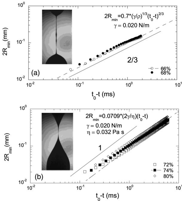
FIG. 2. The minimum neck diameter  $R_{\min}$  of the emulsion vs time, with low and high concentrations of castor oil (powers  $0.67 \pm 0.02$  for  $\phi < 70\%$  and  $0.99 \pm 0.03$  for  $\phi > 72\%$ ).
