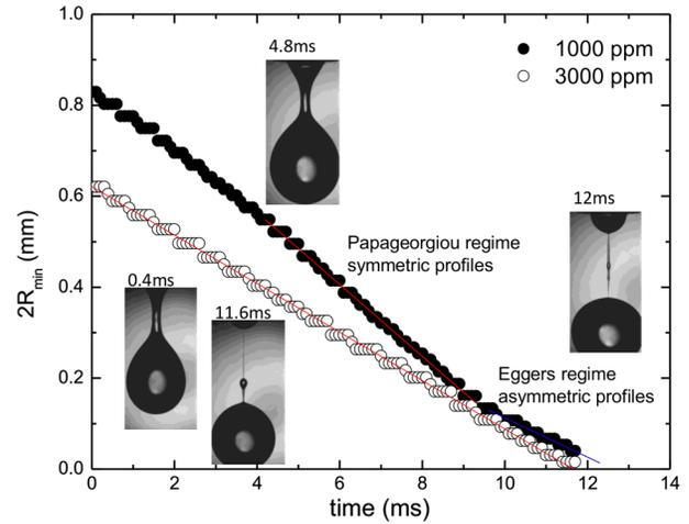
FIG. 5 (color online). Evolution of the diameter  $2R_{\min}$  for low and high concentrations of xanthan in water [1000 ppm (slope  $dR_{\min}/dt = 0.0395$  m/s;  $\eta = 0.128$  Pa s) and 3000 ppm ( $dR_{\min}/dt = 0.0265$  m/s;  $\eta = 0.192$  Pa s)]. Error bars are smaller than the symbols.
