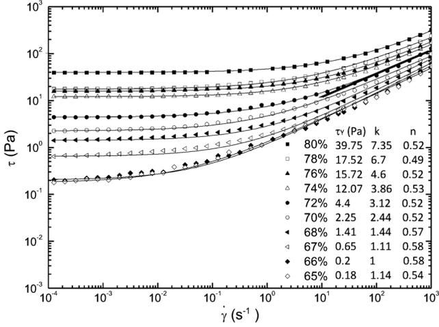
FIG. 1. Yield stress system: shear stress vs shear rate for several volume fractions of castor oil; the shear-thinning exponent is nearly constant,  $n \approx 0.52 \pm 0.04$  (a line of slope  $\frac{1}{2}$  has been added at the right-hand side).
