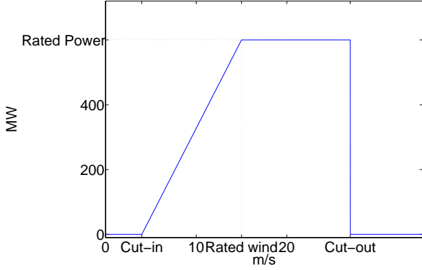
Figure 1. Wind power as function of the wind speed.
