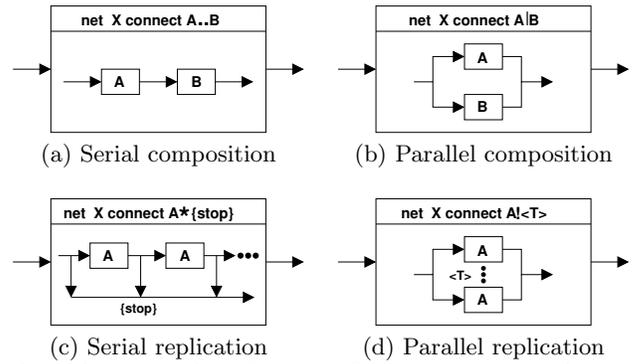
Figure 1: Illustration of the four S-Net network combinators
