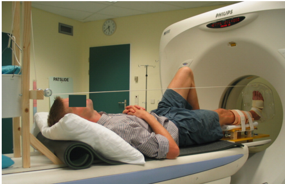
Figure 1 The subject was positioned on the CT table with the right lower leg attached to the supporting platform and with the right foot attached to the footplate. An external load was applied to the footplate to force the otherwise unconstrained foot in the eight extreme positions. Following CT scanning with the foot in the neutral position, scanning was performed for each of the extreme positions separately.
