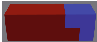
Fig. 3. Imbalanced domain distribution. Both the red and blue parts are assigned to half of the processes. (Color figure online)
