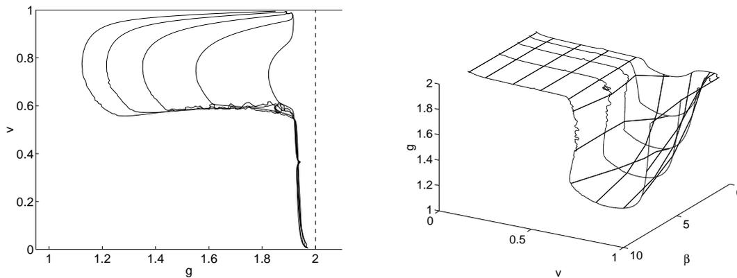
Figure 1: Nonlocal bifurcations before the fundamental equilibrium loses stability: bifurcation curves for several  $\beta$  in a  $(g, v)$ -diagram (left), and the three dimensional bifurcation surface (right).
