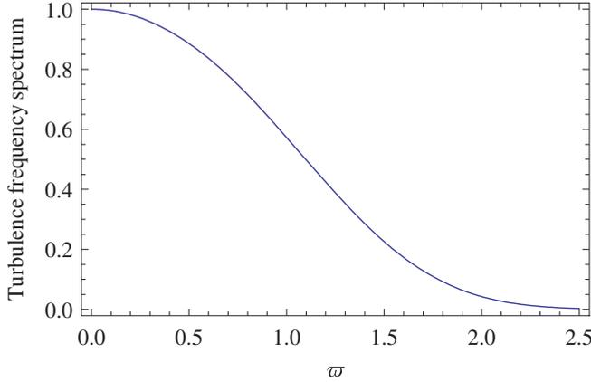
FIG. 1. (Color online) Plot of the self-consistent turbulence frequency spectrum in the scaling range according to Eq. (5.12), normalized at zero frequency, as a function of the nondimensional unswept frequency  $\bar{\omega}$  defined in Eq. (5.13).
