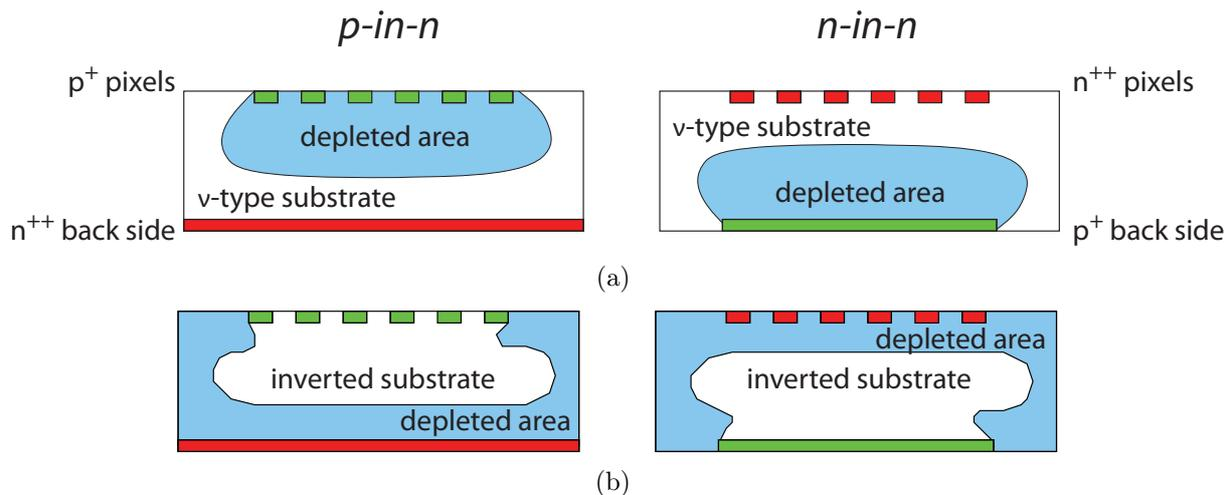
**Figure 2.11: Implanted-junction structures**
