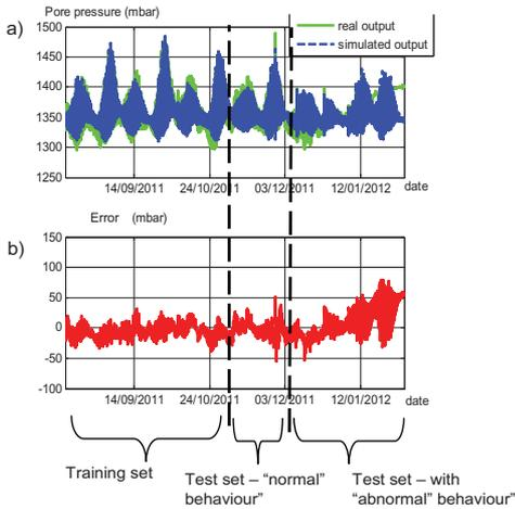
Figure 9. a) Results of one-step forecasting using the *second* linear model; b) Error of one-step forecasting.
