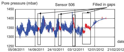
Figure 6. Pore pressure measurements (mbar) from sensor #506. Blue line—raw data, red line—examples of filled in gaps. Extended periods of filled gaps are marked with boxes.
