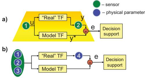
Figure 1. a) Transfer Function (TF) between different sensors; b) Transfer Function (TF) between physical parameters in one sensor module.  $u$  is input sensor signals,  $y$  is output sensor signals,  $y^*$  is model output,  $e$  is output errors.
