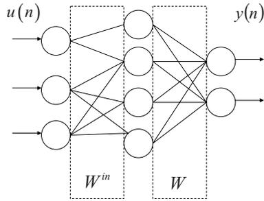
Figure 5. Structure of the three-layered (input, hidden and output layers) feed forward neural network that makes static nonlinear transformation of input  $u(n)$  into output values  $y(n)$ .  $W^{in}$  and  $W$ —matrices of connections (weights) between layers.
