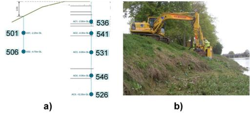
Figure 2. a) Cross-section of Boston dike, circles with numbers show installation of pore pressure sensors; b) Photo of the Boston dike.
