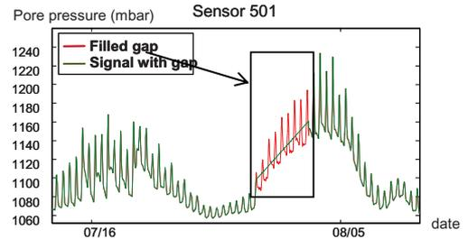
Figure 3. Example of gap filling for pore pressure sensor #501. The "reconstructed" signal is shown in red colour (inside the box). Measurement rate is once every 15 minutes.
