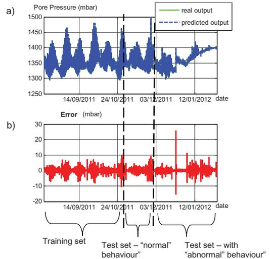
Figure 8. a) Results of one-step forecasting using the *first* linear model; b) Error of one-step forecasting.
