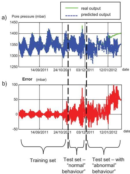
Figure 10. a) Results of one-step forecasting using the FFNN; b) Error of one-step forecasting.
