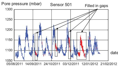
Figure 7. Pore pressure measurements (mbar) from sensor #501. Blue line—raw data, red line—examples of filled in gaps. Extended periods of filled gaps are marked with boxes.
