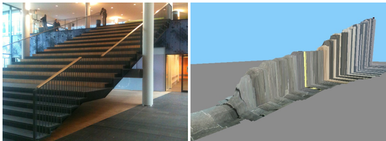
Fig. 10: Photo and map of a large stair at our university which is traversed by the AR.Drone. The depth of each step is 30\text{cm} and the height of each step is 18\text{cm} . The total height of the stair is 480\text{cm} .
