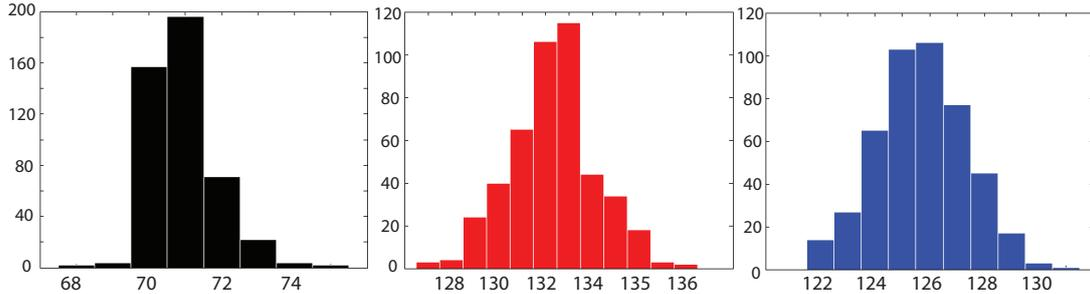
Figure 4.2: Camera noise histogram. The YCrCb values of a single pixel over time are recorded and analyzed using histograms (left - y-channel, middle - Cr-channel, right - Cb-channel)
