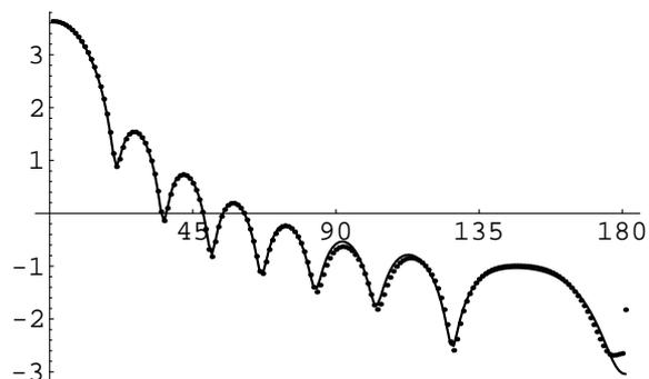
Figure 4: Coupled Dipole simulation (dots) of scattering by a sphere, and Mie calculations (line). The  $S_{11}$  element of the scattering matrix  $S$ , as a function of the scattering angle is shown. The size parameter of the sphere is  $\alpha = 12.6$ , the refractive index is  $m = 1.05$ . The number of dipoles in the CD simulation was 33552, the size of the dipoles was  $\lambda/10$ .
