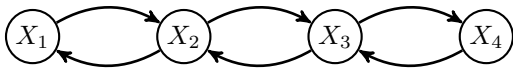
Figure 5: Graph of the structural causal model induced by the mass-spring system for D = 4 .
