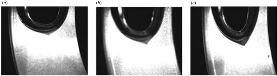
FIGURE 13. Meniscus dynamics for elastic liquid (gap width = 2.3 cm,  $Bo = 117$ ): (a)  $Ca = 1.33$ ,  $Gr = 0.009$ ,  $Wi = 0.74$ ; (b)  $Ca = 1.6$ ,  $Gr = 0.01$ ,  $Wi = 0.89$ ; (c)  $Ca = 2.13$ ,  $Gr = 0.014$ ,  $Wi = 1.18$ .
