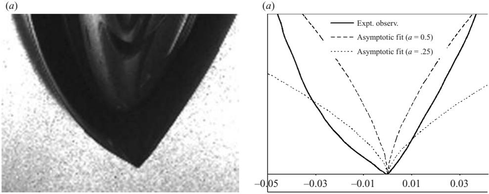
FIGURE 12. (a) Close-up of the two-dimensional sharp interface for  $Ca = 0.913$ ,  $Gr = 0.013$ ,  $Wi = 0.6$  ( $b_{max} = 1.635$  cm,  $Bo = 83$ ). (b) Comparison between the shape of the experimentally observed sharp interface and the asymptotic relation  $y = ax^{2/3}$  for cusps.
