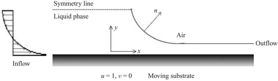
FIGURE 18. Gas-assisted liquid displacement in planar flow geometry.
