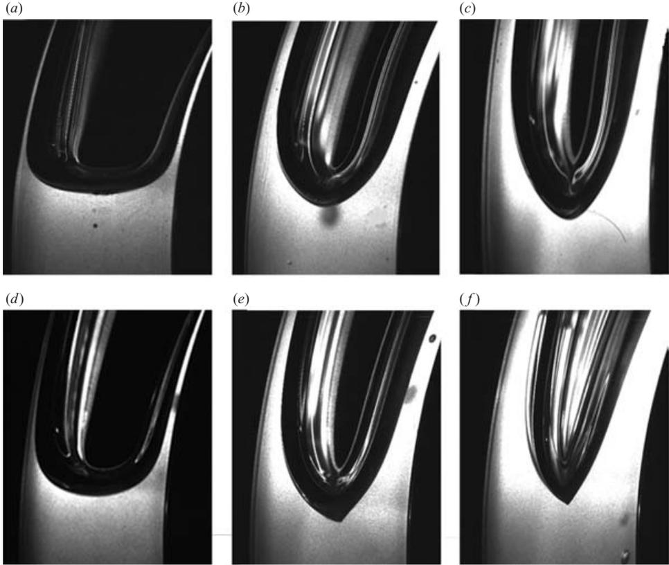
FIGURE 9. Experimentally observed interfacial evolution for both Newtonian (*a-c*) and viscoelastic liquids (*d-f*) ( $b_{max} = 1.635$  cm,  $Bo = 83$ ): (*a*)  $Ca = 0.25$ ,  $Gr = 0.003$ ; (*b*)  $Ca = 0.913$ ,  $Gr = 0.011$ ; (*c*)  $Ca = 1.73$ ,  $Gr = 0.021$ ; (*d*)  $Ca = 0.25$ ,  $Gr = 0.003$ ,  $Wi = 0.2$ ; (*e*)  $Ca = 0.913$ ,  $Gr = 0.011$ ,  $Wi = 0.6$ ; (*f*)  $Ca = 1.73$ ,  $Gr = 0.021$ ,  $Wi = 1.0$ .
