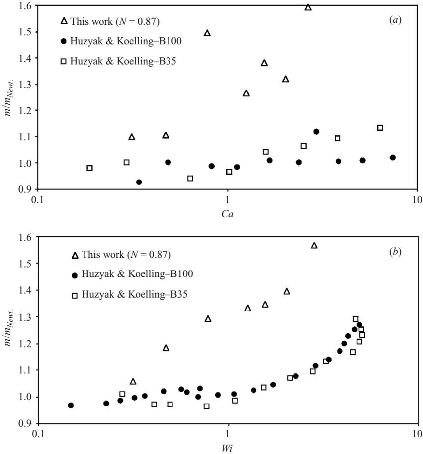
FIGURE 8. Comparison of the reduced fractional coverage,  $m/m_{Newt.}$ , as a function of (a)  $Ca$  and (b)  $Wi$  between data obtained in this study and those measured by Huzyak & Koelling (1997) in a horizontally positioned ( $Bo = 0$ ) capillary tube.
