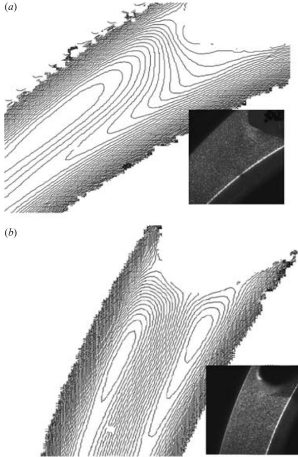
FIGURE 17. Flow streamlines obtained using DPIV for (a)  $b/b_{max} = 0.06$ ,  $Gr = 0.79$  and (b)  $b/b_{max} = 0.6$ ,  $Gr = 0.02$ .
