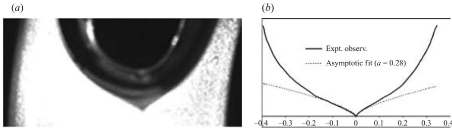
FIGURE 14. (a) Close-up of the two-dimensional sharp interface for  $Ca = 1.6$ ,  $Gr = 0.01$ ,  $Wi = 0.89$ ; ( $b_{max} = 2.3$  cm,  $Bo = 117$ ). (b) Comparison between the experimentally observed cusp and the asymptotic relation  $y = ax^{2/3}$  describing cusps.
