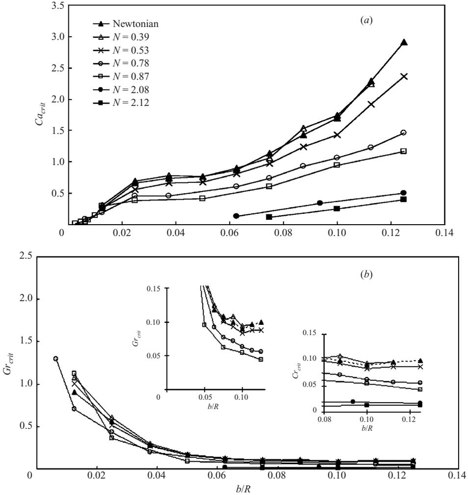
FIGURE 16. Stability curves for both Newtonian and viscoelastic liquids: (a) critical capillary number,  $Ca_{crit}$ , vs. dimensionless gap width,  $b/R$ ; (b) critical gravity number,  $Gr_{crit}$ , vs. dimensionless gap width,  $b/R$ .
