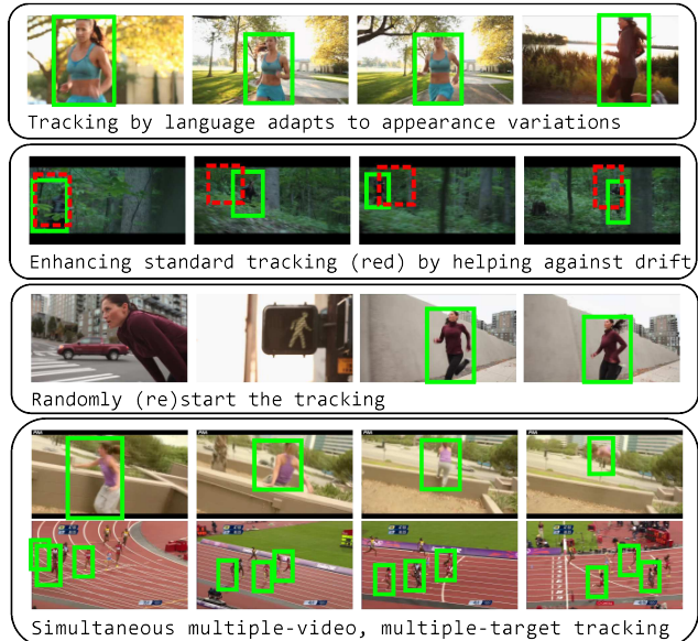
Figure 1: Tracking by natural language specification allows for a novel type of human-machine interaction in object tracking. It enhances standard trackers by helping them against drift. It also opens up opportunities for new applications like random start tracking, for example when the target is lost, or simultaneous multiple-video tracking.
