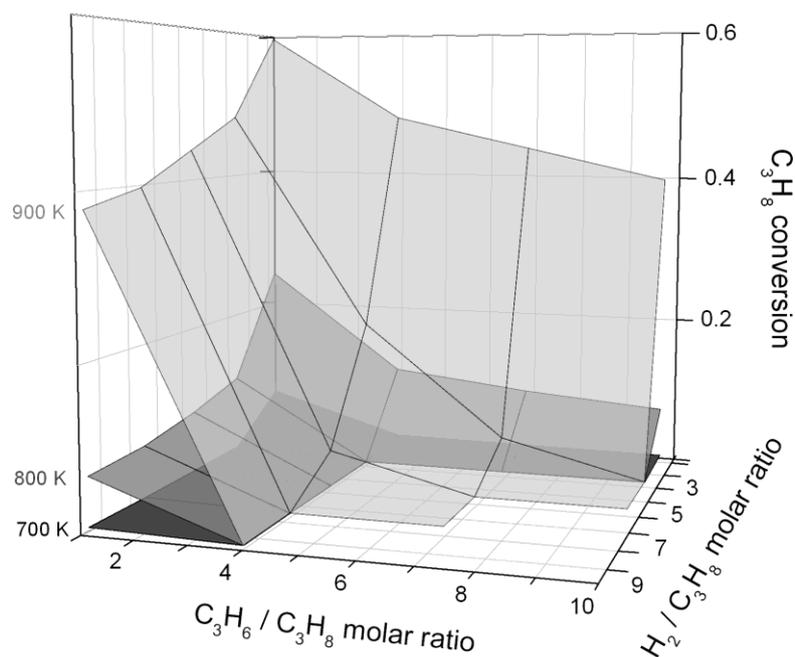
**Figure B2:** Propane dehydrogenation equilibrium conversion (Z-Axis) as a function of the ratios propylene/propane (X-Axis, left-to-right) and hydrogen/propane (Y-Axis, front-to-back). Each surface represents data calculated at different temperatures (see eqns. (B.6) and (B.7)).
