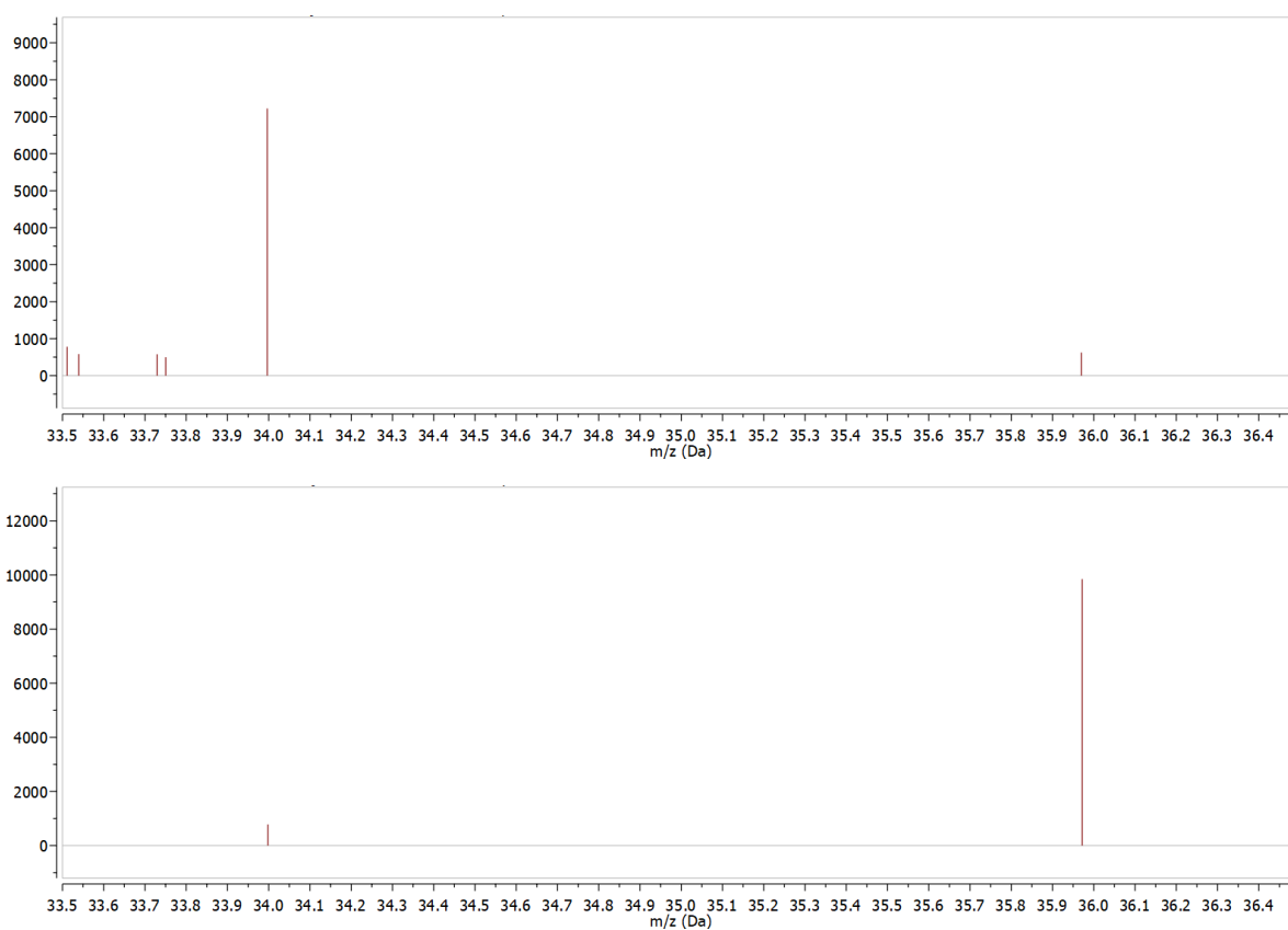
Supporting Information Figure S3. MS spectrum of the oxygen evolution reaction in a 0.10 M acetate buffer using 0.10 M Oxone with ~80% O 18 labeled water at a pH of 5.0 without (top) and with 0.10 mM of nickel complex 1 (bottom) .
