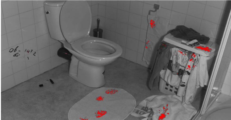
Figure 3.10. Greyscale image (one wavelength band of the hypercube), overlaid with red pixels showing identified blood stains at a threshold R^2 of 0.98.
