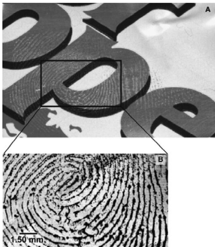
Figure 2.7. Cut and flattened Dr. Pepper's soda can with fingermark deposit. (A) Soda can imaged by a document scanner. B) Infrared image of the outlined area obtained by plotting the band intensity at 9842 nm (1016 \text{cm}^{-1} ). Reprinted from Journal of Forensic Sciences , 52/1, Nicole J. Crane, Edward G. Bartick, Rebecca Schwartz Perlman, Scott Huffman, Infrared Spectroscopic Imaging for Noninvasive Detection of Latent Fingerprints , 48-53, Copyright (2012), with permission from John Wiley and Sons 28 .
