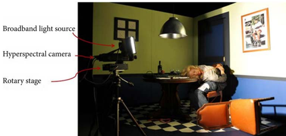
Figure 2.5. Hyperspectral imaging system at a simulated crime scene.
