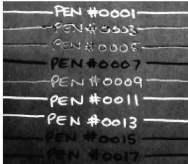
Figure 2.10. Third principal component of blue ink set, indistinguishable with the human eye. Reprinted from Talanta , 67/2, Gemma Payne et al, Visible and near-infrared chemical imaging methods for the analysis of selected forensic specimens, 334–344 Copyright (2012), with permission from Elsevier 51 .
