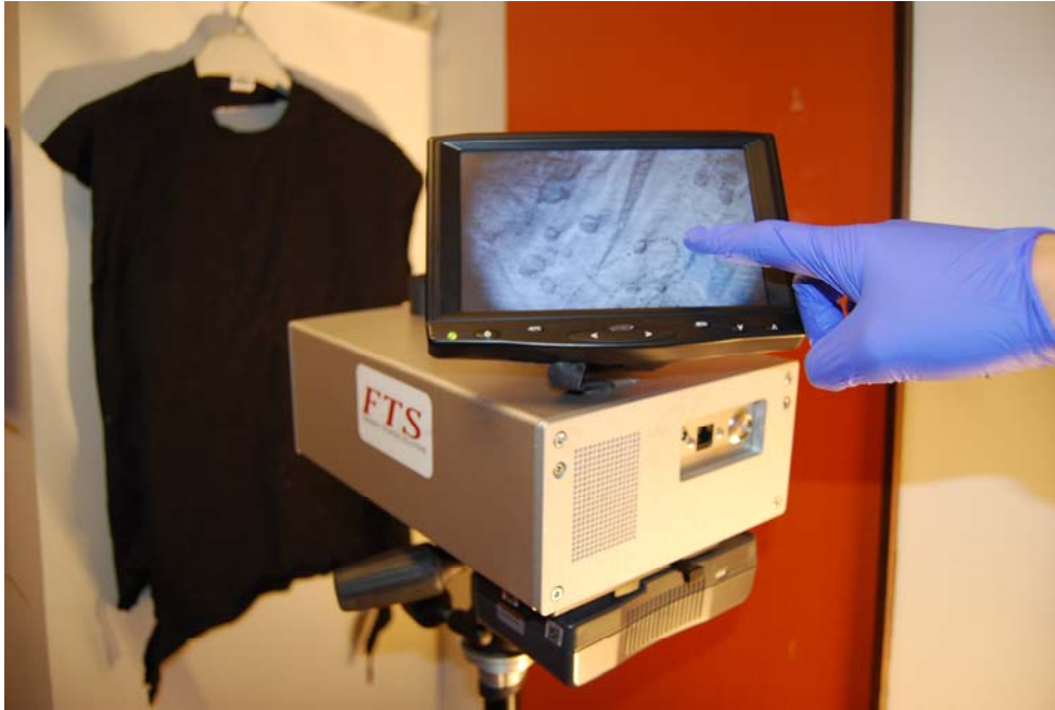
Figure 6.1. Custom made wireless hyperspectral imaging system, consisting of a liquid crystal tuneable filter, a CCD camera, a lens, a built-in acquisition board, computer, a battery, and a touch screen. A single wavelength band is shown on the live view of the camera.
