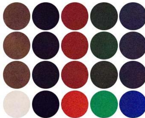
Figure 7.1. Photographs of blood stains on white, black, red, green and blue cotton and corresponding plain reference samples (bottom row).
