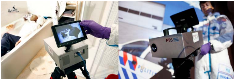
Figure 9.4. Photographs of a hyperspectral imaging system at a simulated crime scene.
