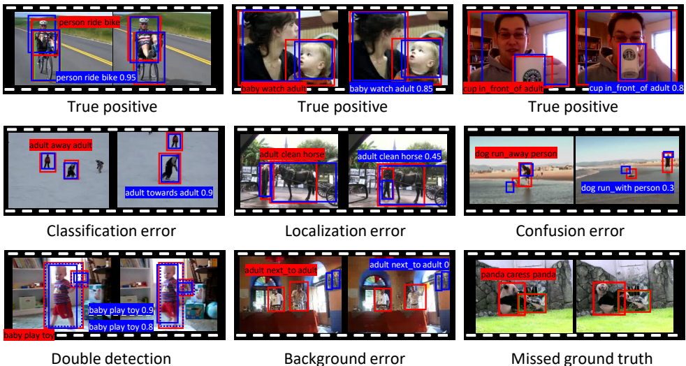
Figure 2: Video relation detection examples of true positives and the six error types from Table 1. Red boxes indicate ground truth and blue boxes specify predictions. The number in the blue box is the vIoU between the detection and the ground truth. The dashed boxes in double detection represent the best mapped prediction to this ground truth. To match a prediction to a ground truth is difficult and many factors could influence the final performance.
