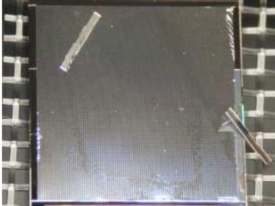
Figure 4. The dykes that support the grid along the perimeter are the weak point of the structure at cold temperature ( \sim 140 K in this test). Under thermal stress they lose adhesion to the underlying protection layer and the tension of the grid rips them off.
