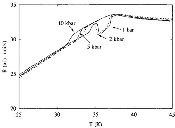
Fig. 2. Temperature dependences of the resistivity  $\rho$  (for the current  $\parallel c$ -axis) in UNiGa in the temperature range of several magnetic phase transitions measured under different external pressures.
