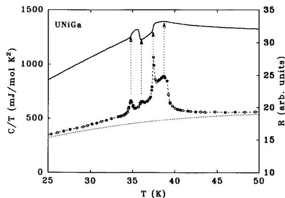
Fig. 1. Temperature dependences of the specific heat divided by temperature ( $C/T$ ) (open symbols) and of the resistivity  $\rho$  for the current  $\parallel c$ -axis (full line) in UNiGa in the temperature range of several magnetic phase transitions.
