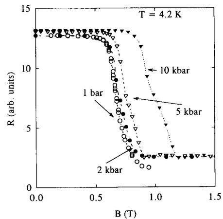
Fig. 6. Field dependences of the resistivity  $\rho$  (for the current  $\parallel c$ -axis) in UNiGa in the temperature range of several magnetic phase transitions measured under different external pressures.
