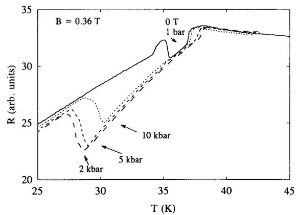
Fig. 4. Temperature dependences of the resistivity  $\rho$  (for the current  $\parallel c$ -axis) in UNiGa in a magnetic field of 0.36 T ( $B \parallel c$ -axis) in the temperature range of several magnetic phase transitions measured under different external pressures.
