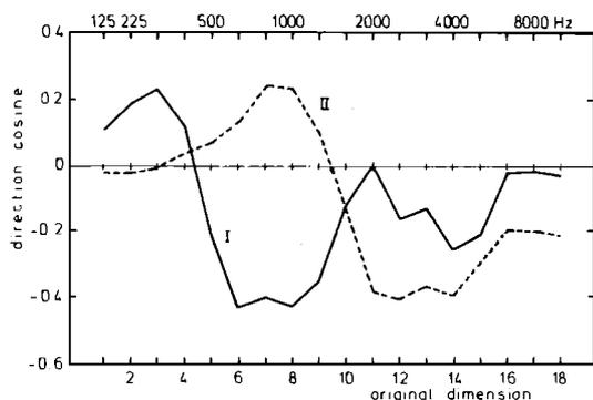
FIG. 7. Direction cosines between these axes in the maximally discriminating plane, related to best match with the  $\log F_1$ - $\log F_2$  plane, and the original 18 dimensions representing the levels below overall SPL in 18  $\frac{1}{3}$ -oct bands.
