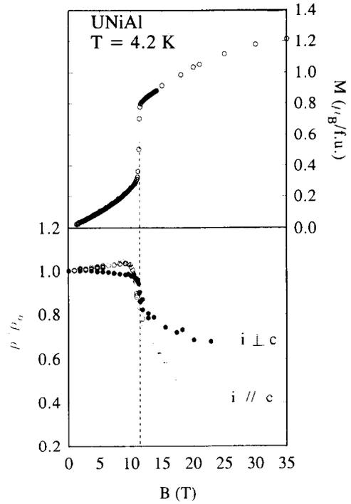
Fig. 4. (upper part) Magnetization curve of the UNiAl single crystal at 4.2 K for  $B \parallel c$ . (lower part) Magnetic field dependence of the relative electrical resistivity ( $\rho_0$  = the value at  $B = 0$  T) of the UNiAl single crystal at 4.2 K for  $B \parallel c$ ,  $i \parallel c$  and  $i \perp c$ .
