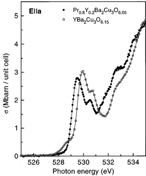
FIG. 7. O  $1s$  absorption spectra of the O atoms in the plane for oxygen-deficient  $\text{Pr}_{0.8}\text{Y}_{0.2}\text{Ba}_2\text{Cu}_3\text{O}_{6.05}$  and  $\text{YBa}_2\text{Cu}_3\text{O}_{6.15}$ . In both cases a distinct UHB is observed. The onset of the UHB for  $\text{Pr}_{0.8}\text{Y}_{0.2}\text{Ba}_2\text{Cu}_3\text{O}_{6.05}$  is downshifted by  $\approx 0.35$  eV.
