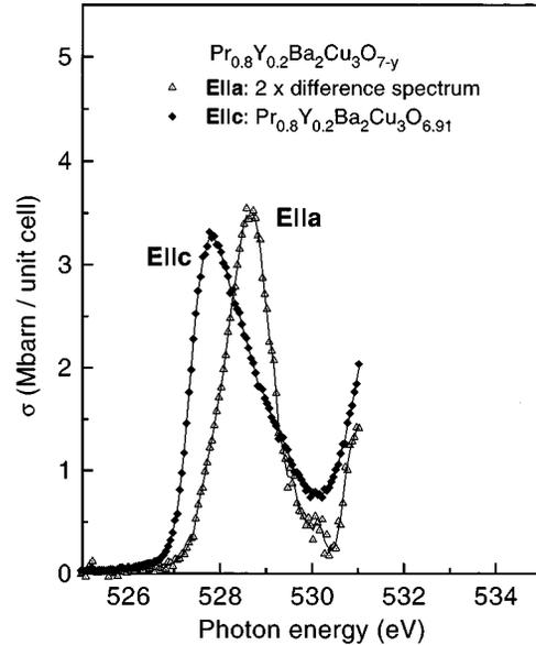
FIG. 12. Comparison of the planar difference spectrum  $2(\text{Pr}_{0.8}\text{Y}_{0.2}\text{Ba}_2\text{Cu}_3\text{O}_{6.91}-\text{Pr}_{0.8}\text{Y}_{0.2}\text{Ba}_2\text{Cu}_3\text{O}_{6.05})$  and the  $\mathbf{E}\parallel c$  spectrum of  $\text{Pr}_{0.8}\text{Y}_{0.2}\text{Ba}_2\text{Cu}_3\text{O}_{6.91}$ . The area enclosed by both curves constitutes an upper limit for *isotropic* FR states.
