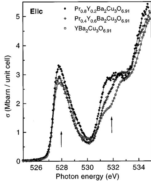
FIG. 6.  $\mathbf{E}\parallel c$  spectra of  $\text{Pr}_x\text{Y}_{1-x}\text{Ba}_2\text{Cu}_3\text{O}_{6.91}$  ( $x=0.8, 0.4, 0.0$ ). For  $\text{YBa}_2\text{Cu}_3\text{O}_{6.91}$  the complete peak at 528 eV is ascribed to the apical oxygen atoms while for  $\text{Pr}_{0.8}\text{Y}_{0.2}\text{Ba}_2\text{Cu}_3\text{O}_{6.91}$  the peak also contains contributions from the FR state.
