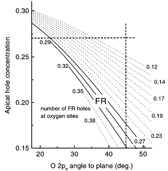
FIG. 13. Test of the Fehrenbacher-Rice model. The apical hole concentration is depicted as a function of the rotation angle of the O(2,3)  $2p_\pi$  orbitals, as calculated from Eq. (3) (in the text). NEXAFS results of this work are incorporated (see text).
