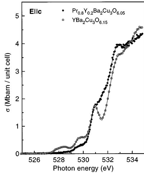
FIG. 8. O  $1s$  absorption spectra of  $\text{Pr}_{0.8}\text{Y}_{0.2}\text{Ba}_2\text{Cu}_3\text{O}_{6.05}$  and  $\text{YBa}_2\text{Cu}_3\text{O}_{6.15}$  for polarization parallel to the  $c$  direction. For both samples an UHB is absent since the UHB has predominantly planar character.
