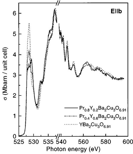
FIG. 2. O 1s absorption spectra of  $\text{Pr}_{0.8}\text{Y}_{0.2}\text{Ba}_2\text{Cu}_3\text{O}_{6.91}$ ,  $\text{Pr}_{0.4}\text{Y}_{0.6}\text{Ba}_2\text{Cu}_3\text{O}_{6.91}$ , and  $\text{YBa}_2\text{Cu}_3\text{O}_{6.91}$  for polarization  $\mathbf{E}||b$ . The data are shown in the entire energy range recorded. Above 540 eV, the cross sections are independent of the Pr concentration.
