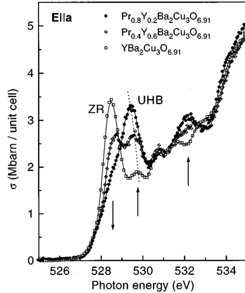
FIG. 3. Comparison of the O 1s absorption spectra of Pr<sub>0.8</sub>Y<sub>0.2</sub>Ba<sub>2</sub>Cu<sub>3</sub>O<sub>6.91</sub>, Pr<sub>0.4</sub>Y<sub>0.6</sub>Ba<sub>2</sub>Cu<sub>3</sub>O<sub>6.91</sub>, and YBa<sub>2</sub>Cu<sub>3</sub>O<sub>6.91</sub> for  $\mathbf{E}||a$ . Upon Pr substitution, the upper Hubbard band increases strongly at the expense of the ZR state.
