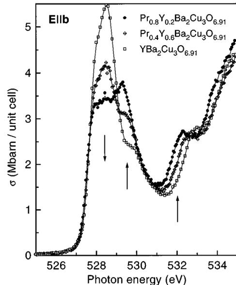
FIG. 4. O 1s absorption spectra of Pr<sub>0.8</sub>Y<sub>0.2</sub>Ba<sub>2</sub>Cu<sub>3</sub>O<sub>6.91</sub>, Pr<sub>0.4</sub>Y<sub>0.6</sub>Ba<sub>2</sub>Cu<sub>3</sub>O<sub>6.91</sub>, and YBa<sub>2</sub>Cu<sub>3</sub>O<sub>6.91</sub> for  $\mathbf{E}||b$ . For  $\mathbf{E}||b$  an analogous trend is observed as for the  $\mathbf{E}||a$  spectra.
