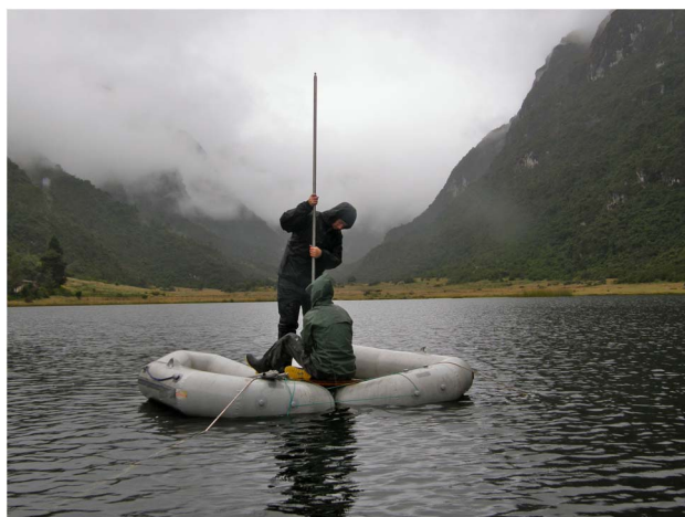
Figure 2. (color online) A core being raised using a Colinvaux-Vohnout piston sampler from a raft of inflatable boats at Lake Llaviucu (also called Surucucho) in June 2010. This lake had previously been cored by Colinvaux's team in 1988 (Colinvaux et al., 1997).
