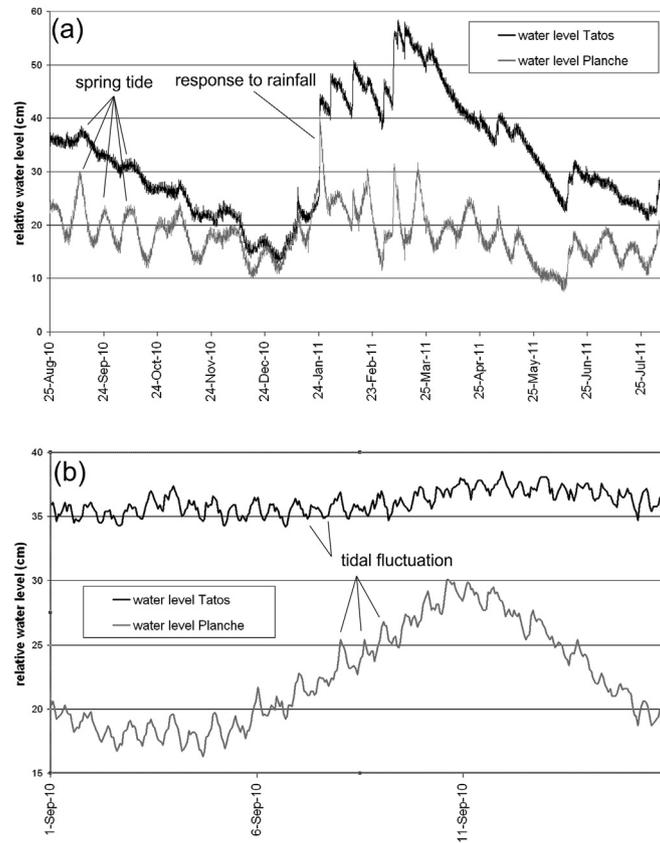
Fig. 7. Water level fluctuations measured in Tatos and Planche showing responses to sea level changes and rainfall event for periods of (a) 1 year and (b) 15 days.
