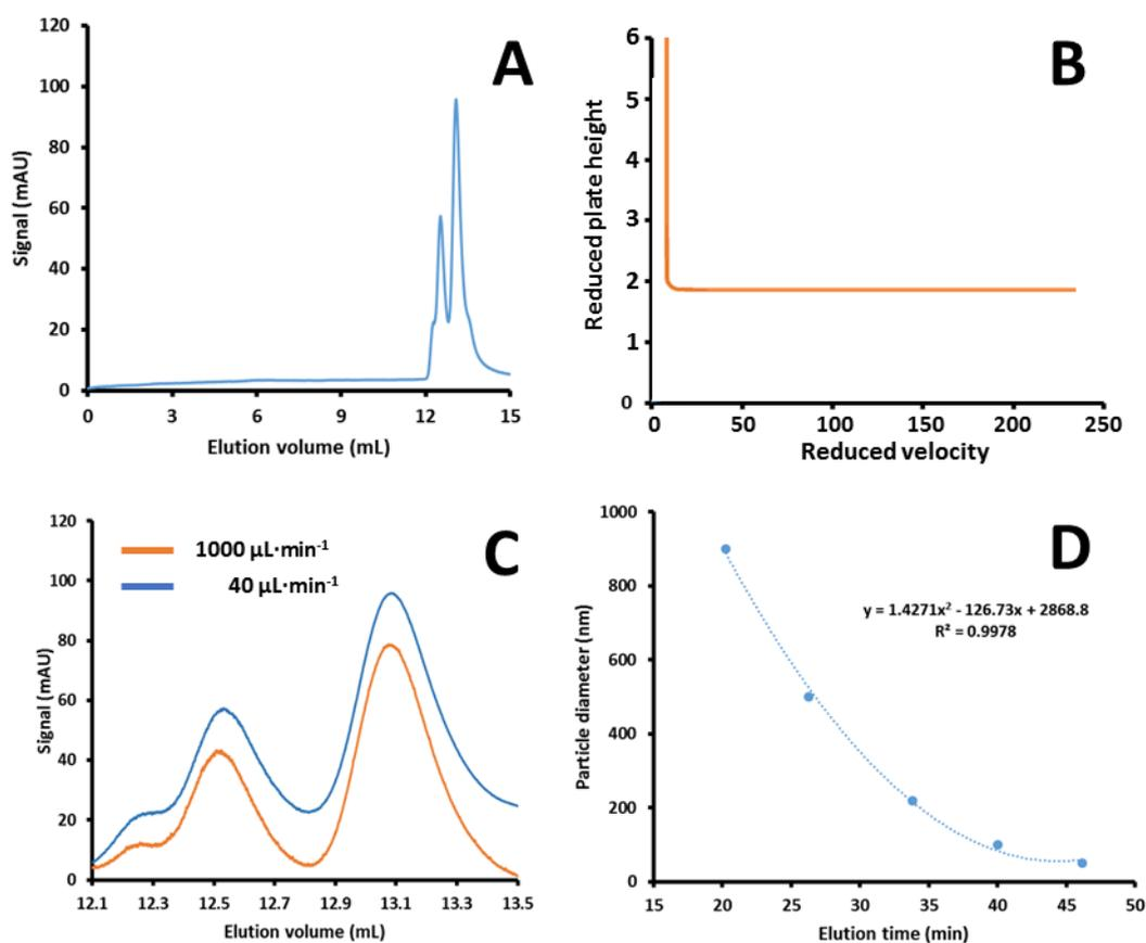
**Figure S-1:** A: Chromatogram of the separation of a mixture of PS nanoparticles (900 nm, 498 nm, 100 nm and 50 nm) by HDC using System A. B: Theoretical van Deemter plot for nanoparticles. C: Overlay of section of HDC chromatogram obtained using System A at 1 mL $\cdot$ min $^{-1}$  and 40  $\mu\text{L}\cdot$ min $^{-1}$  following a flush program as described in the Analytical Methods section of the article. D: Calibration curve of the HDC separation using the flush program.
