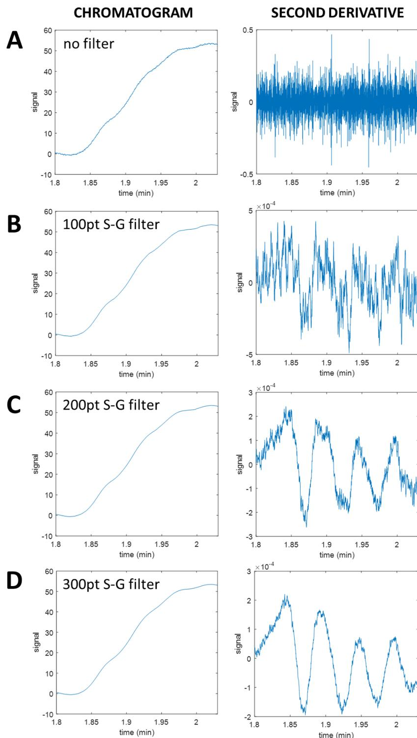
**Figure S-5:** Chromatogram signal (left) with the corresponding second derivative (right) using A) no filter, B) 101, C) 201 and D) 301 points wide Savitsky-Golay (S-G) smoothing filter. While needed to remove the disturbing background noise from the signal to allow a proper second derivative to be taken, the S-G filters do not remove the features of interest from the chromatogram.
