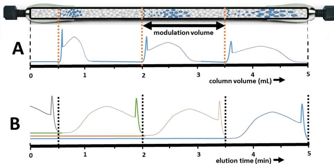
**Figure S-2:** Theoretical sketch illustrating the principle of overlapping injections. A: The modulation time is adapted such that the sample zones of subsequent injections do not overlap. B: The observed chromatogram after the second dimension reflects exclusively the SEC domain of the separation, provided that none of the sample components are adsorbed on the column. Note: The three SEC columns coupled together for our study are shown here as a single column for simplicity.
