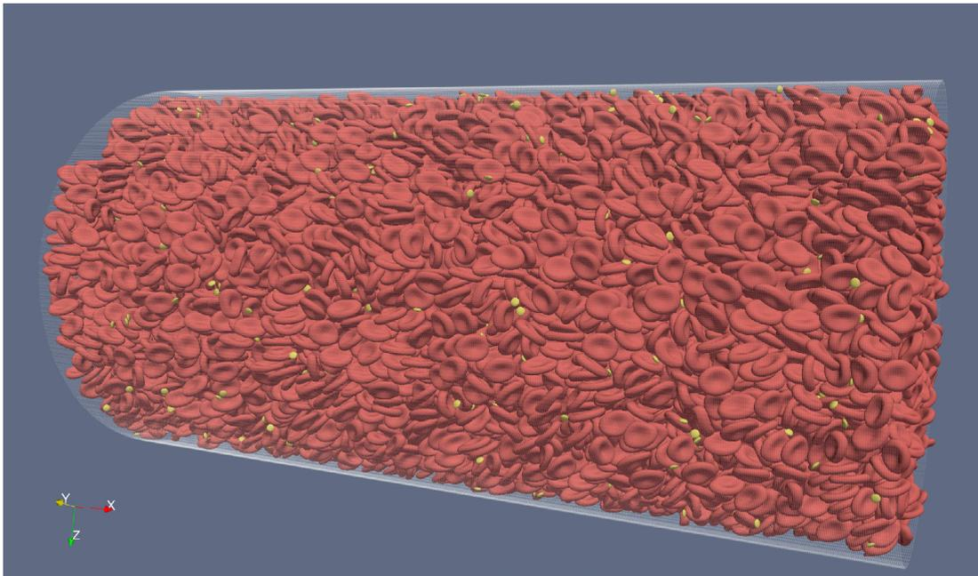
Figure 3: Simulation of cellular flow inside a small vessel with the diameter of  $128\mu\text{m}$  at a hematocrit level of 46%.
