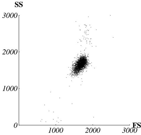
Figure 2: An example of a two parameter scatterplot for a large number of polystyrene spheres with a mean diameter of  $1.98 \mu\text{m}$ , measured with a FlowCytometer. The wavelength was  $0.6328 \mu\text{m}$ . Every dot represents a single sphere, the value of the x-coordinate is the intensity of the forward scattered light, the value of the y-coordinate is the intensity of the sideward scattered light. The intensities are in arbitrary units.
