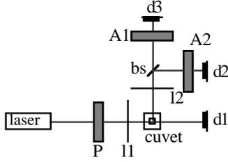
Figure 1: Schematic drawing of the optical system of the FlowCytometer. The laser beam is focussed by lens **I1** on a cell, flowing through the cuvet. The incident beam is polarized by means of the polarizer **P**. The intensity of the forward scattered light is measured by detector **d1**, the sideward scattered light is focussed by lens **I2** on detectors **d2** and **d3**, **bs** is a beamsplitter. The side scattering signals are passed through two different analyzers **A1** and **A2**.
