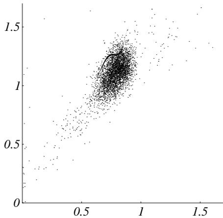
Figure 4: The normalized experimental and theoretical ( $s_{11}+s_{12}$ ,  $s_{11}-s_{12}$ ) scatterplot for polystyrene spheres with a mean diameter of  $1.98 \mu\text{m}$ . The horizontal axis is the  $s_{11}+s_{12}$  signal in the sideward direction, the vertical axis is the  $s_{11}-s_{12}$  signal in the sideward direction.
