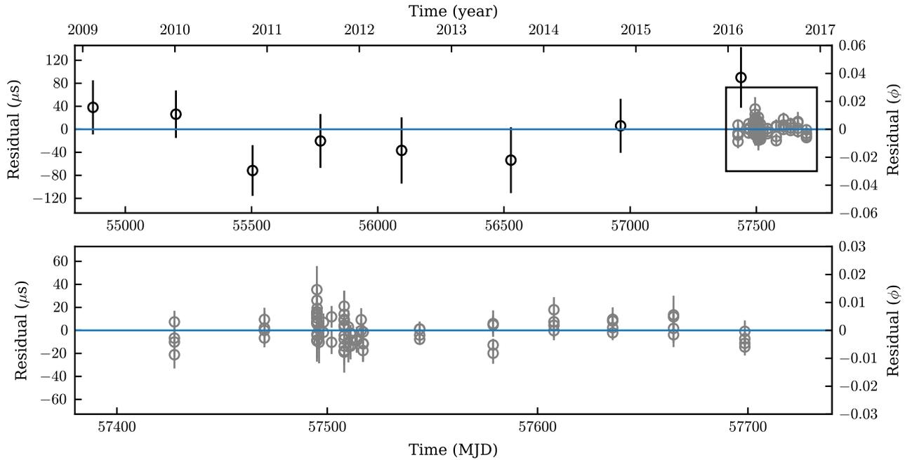
**Figure 4.** Timing residuals for PSR J1552+5437 as a function of time. The model is depicted with a blue line, the *Fermi* TOAs with black circles, and the LOFAR TOAs with gray circles. The lower panel is a magnification of the upper panel, showing only the LOFAR TOAs.
